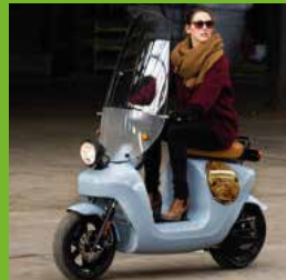
Scooter made from bioplastic composite
